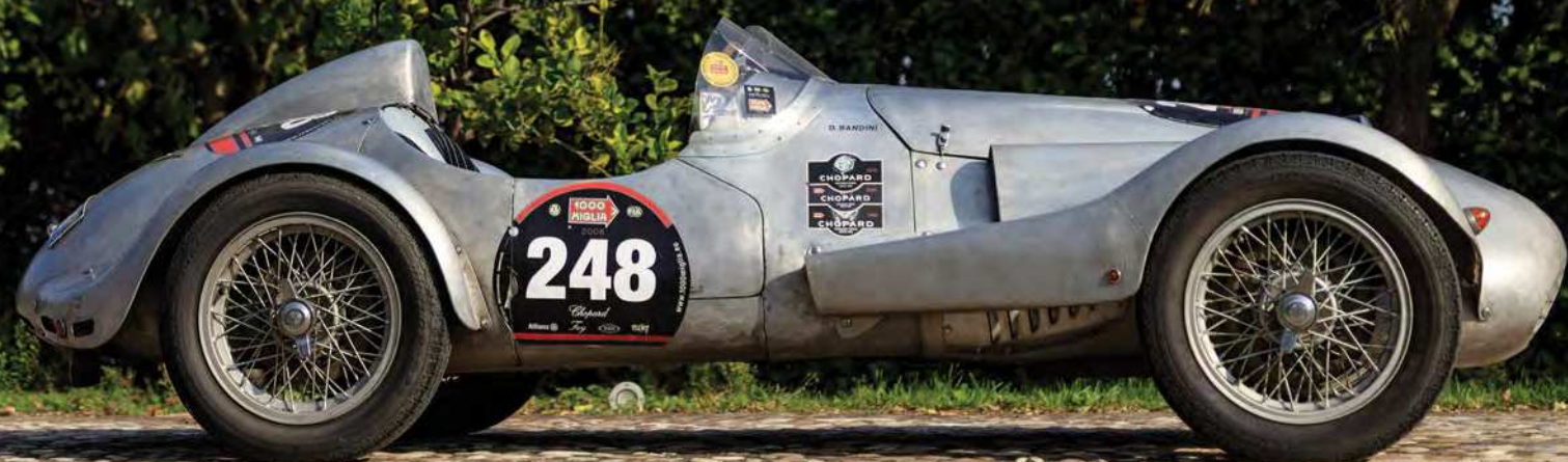
ABOVE: Bandini 750 used a Crosley-based 747cc engine fitted with a twin-cam head. BELOW: Formula Junior 1100 racer from 1960
